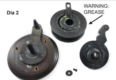
**2.** Separate the 3 parts of the winch. The winch contains a lot of grease so please be careful not to get any on your clothes. You might want to clean it off around the barrel, where the rope is going to run at this stage if you prefer. You now have access to the wooden back board.
