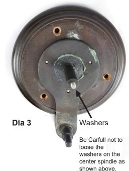
**3.** Screw the wooden back board into position on your wall using the screws provided and the 3 holes in the board itself. Screw it to the wall with the location arm at the bottom as shown in Dia 3.
